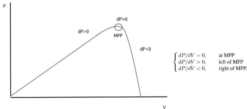
Fig.6. PV array power curve.
