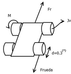
Fig.2. Mechanical scheme of the robot.
