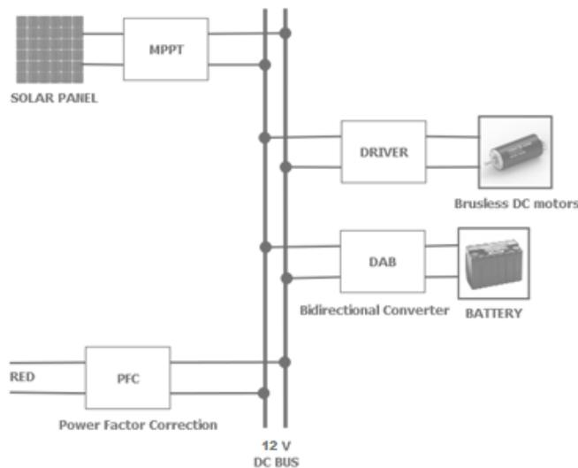
Fig.3. Power system scheme
