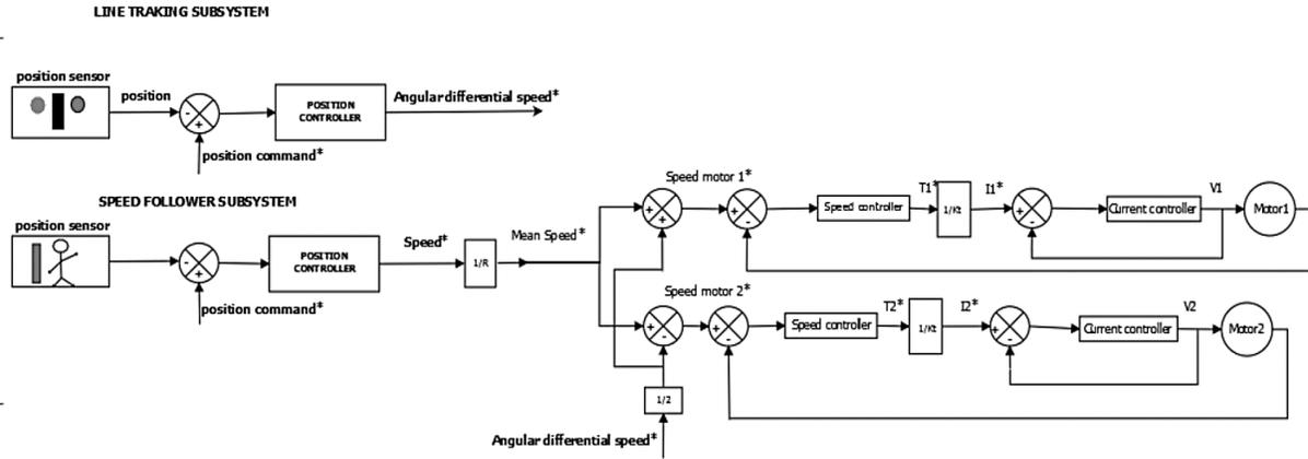
Fig.8. Control system scheme.
