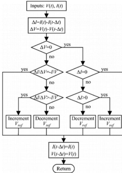
Fig.7. Open loop incremental conductance algorithm [2]
