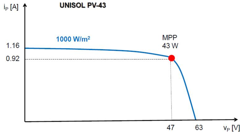
Fig.7. Solar panel output with maximum radiation
